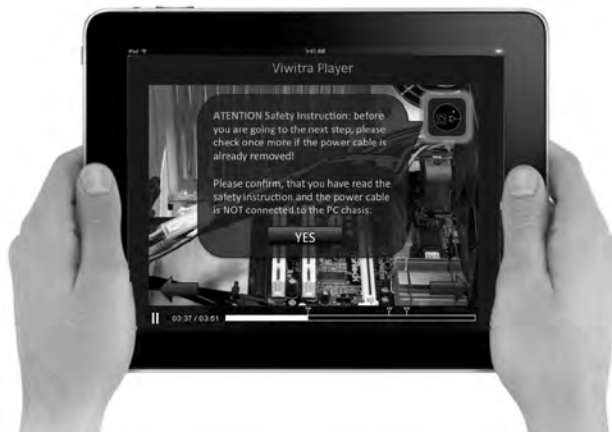
Figure 6: Draft of the VIWITRA player with the danger information and confirmation functionality for removing the power cable
